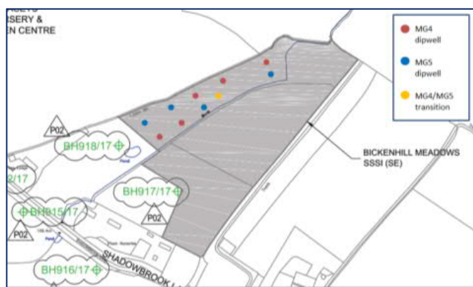
Figure 12a. Locations of dipwells installed in the wet meadow field at the SE SSSI unit
